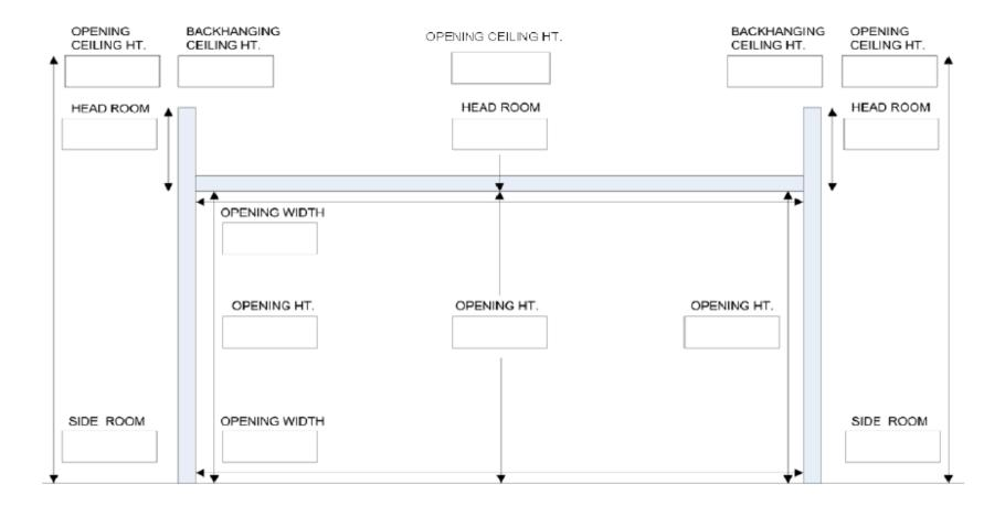
Shown above are the important dimensions we need to know to properly size and quote your new garage door. Opening dimensions are finished dimensions (as opposed to rough opening dimensions).
